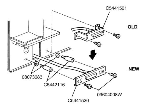
3. To enable the installation of the kit for the RN925, some new parts have been added as "for PART 1D" (see page 6). Also, the cable going to the rear of the machine from the interface board has been lengthened by 100 mm (P/N - C5441500 has been changed to P/N - C5441520) since the old cable was too short for the RN925. (See page 4. The new cable is used for all models.) The new ROM is also required (see the next page).
